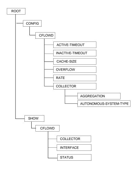
**Figure 35: Cflowd Command Structure**
